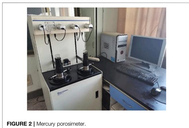
**FIGURE 2** | Mercury porosimeter.
