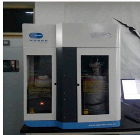
**FIGURE 1** | Hsorb-2600 high-temperature and high-pressure gas adsorbent instrument.
