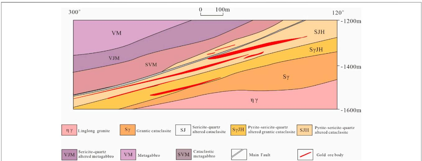
FIGURE 3 | Simplified cross-section of the Zhaoxian gold deposit.
