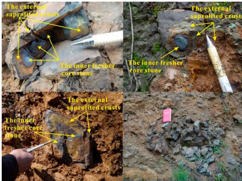
**FIGURE 17** | Basaltic rocks present the structure the structure of soil sandwiching rock due to severe weathering.
