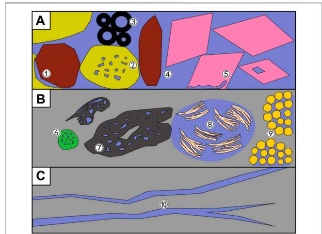
**FIGURE 2** | Key components of shale microstructure and their relationships with pores. **(A)** Grain laminae: (1) pores at the edge of rigid grains, (2) moldic pores, (3) pores within fossil bodies, (4) pores between grains and crystals, and (5) dissolution-rim pores; **(B)** Organic-matter aggregates: (6) pores within peloids or pellets, (7) organic-matter pores, (8) pores between or within clay platelets, and (9) intercrystalline pores within pyrite framboids; and **(C)** (10) fracture.
