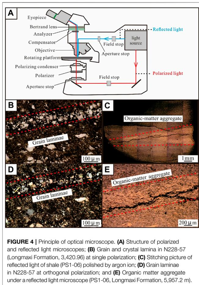
**FIGURE 4 |** Principle of optical microscope. **(A)** Structure of polarized and reflected light microscopes; **(B)** Grain and crystal lamina in N228-57 (Longmaxi Formation, 3,420.96) at single polarization; **(C)** Stitching picture of reflected light of shale (PS1-06) polished by argon ion; **(D)** Grain laminae in N228-57 at orthogonal polarization; and **(E)** Organic matter aggregate under a reflected light microscope (PS1-06, Longmaxi Formation, 5,957.2 m).
