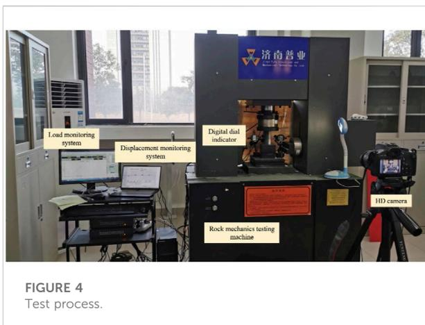
and saved automatically using a computer. The whole stress–strain curve of uniaxial compression concrete specimens with holes of different diameters could be obtained.
