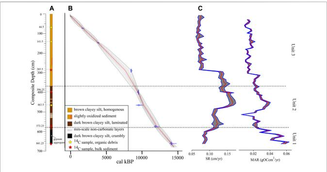
FIGURE 2 | (A) General stratigraphy and (B) age-depth model of the sediment core, based on radiocarbon dating of 7 samples, shown as green/yellow stars (see details in **Table 1**). (C) Inferred sedimentation and mass accumulation rate (SR and MAR) curves along the core, based on the age-depth model.
