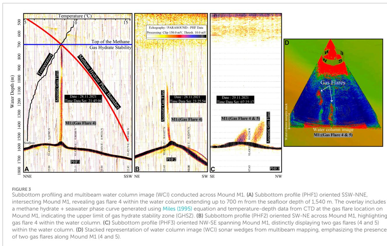
orientations (PHF1 (SSW-NNE), PHF2 (SW-NE), and PHF3 (SE-NW) in Figure 2B), illustrate flare characteristics (Figures 3A–C). The upper limit of hydrate stability, derived for methane and seawater (Miles, 1995) and CTD temperature-depth information, is about 700 m, which matches with the flare termination (Figure 3A).
