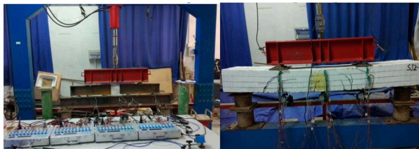
FIGURE 4 Experimental loading diagram for test beams.
