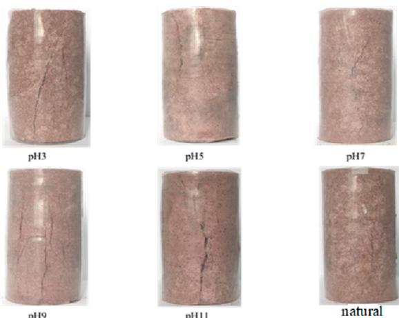
FIGURE 6 Deformation and failure diagram of sandstone under uniaxial compression.
