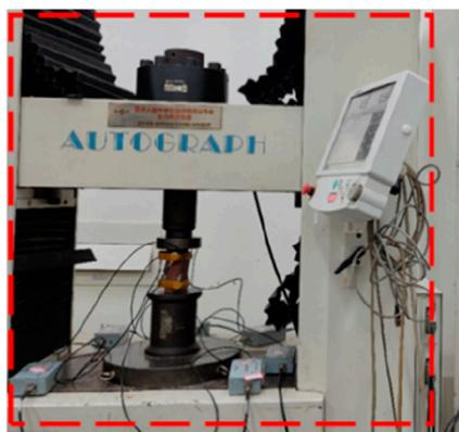
FIGURE 4 AG-250kNIS electronic precision material testing machine.
