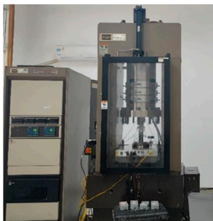
FIGURE 5 MTS815 test equipment diagram.
