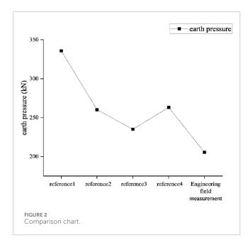
compared with the real-world data. It is shown that the reference 3 is approaching actual engineering values. That is to say the reference 3 is much more reasonable compared with another three references. Currently, the research assumes the retaining structure to be rigid, and the earth pressure law under the condition of the interaction between the retaining structure and the soil and the coordinated deformation can be further studied.
