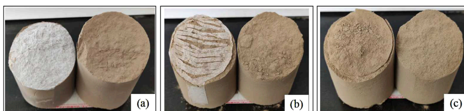
FIGURE 5 The joint surfaces of different materials. (a) Single-layer paper. (b) Single-layer paper with a mesh pattern. (c) Single-layer rice paper.
