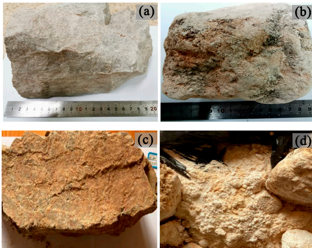
FIGURE 1 Typical photos of dolomite with different sanding grade (a) slight sanding dolomite, (b) moderate sanding dolomite, (c) strong sanding dolomite, (d) severe sanding dolomite.
