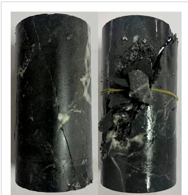
FIGURE 3 Medium weathering limestone sample of experimental test.
