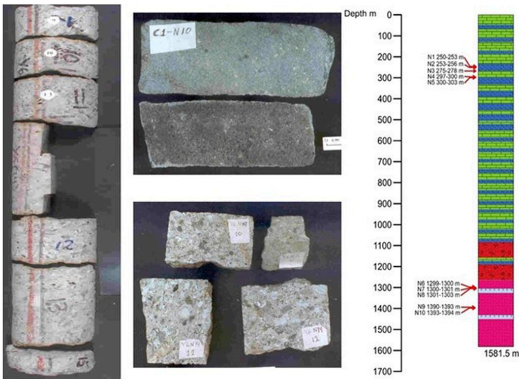
FIGURE 7 Core images for the Yucatan-6 borehole Y6–N14 interval and the Chicxulub-1 borehole C1–N10 interval.
