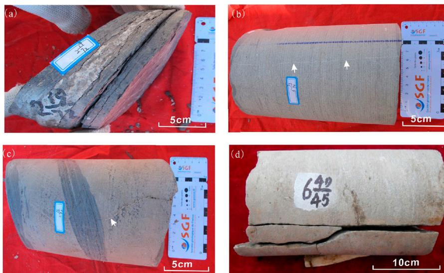
**FIGURE 4** Core samples photographs in the study area. **(A)** Low-angle bedding-parallel oblique fracture; **(B)** High-angle vertical structural fractures with calcite-filled fissure; **(C)** Structural fractures extending along the sandstone and terminating at a mudstone interlayer; **(D)** High-angle vertical structural fracture.
