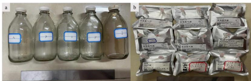
FIGURE 4 Collect gas samples. (a) was used to obtain 5 groups of bagged samples by drainage and gas collection method, (b) was used to obtain 5 groups of bagged samples by drainage and gas collection method. B is the pre-vacuum sampling method to obtain 9 groups of bagged samples.
