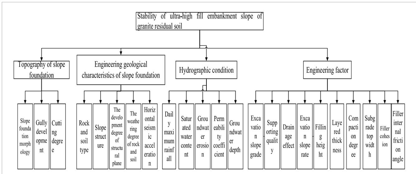
FIGURE 2 Comprehensive evaluation indicator set of embankment slope stability.
