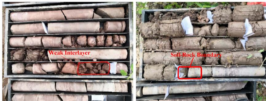
FIGURE 3 Boreholes reveal the weak interlayers and the soil-rock boundary.
