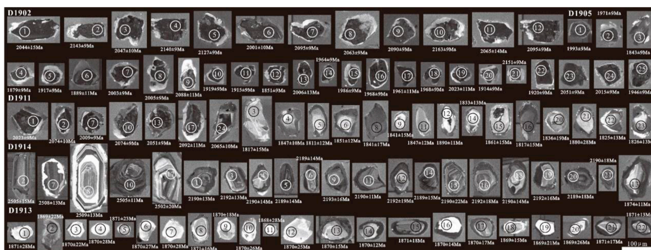
FIGURE 3 Cathodoluminescence (CL) images of the selected zircons from the mafic rocks in the Lieryu Formation. The circles on zircons represent analyzed spots.
