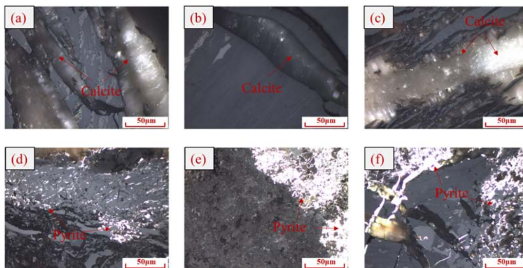
FIGURE 6 Characteristics of the mineral under an optical microscope in oil-immersed reflected light: (a–c) calcite, (d–f) pyrite.
