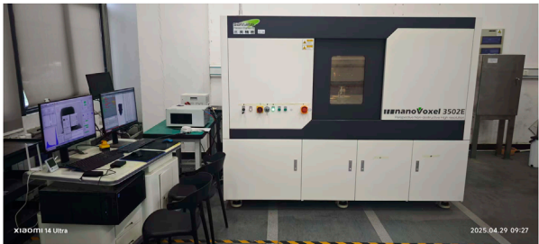
FIGURE 7 The Nano Voxel 3502E open tube transmission CT system.
