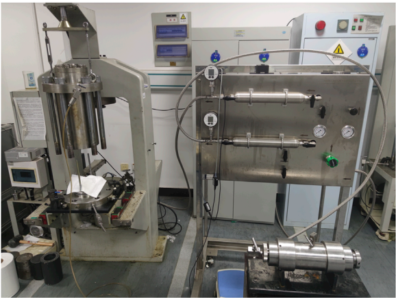
FIGURE 5 The THMC multi-field coupled seepage test system.
