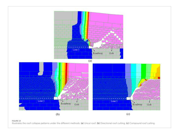
cutting effectively fragmented the long cantilever beam into shorter segments. Simultaneously, the action of non-directional roof cutting induced sufficiently complete roof collapse within the gob area. The resulting collapsed gangue fully filled the gob, thereby providing effective filling support to the overlying gob roof. Consequently, deformation and damage in the roadway surrounding rock were substantially improved.
