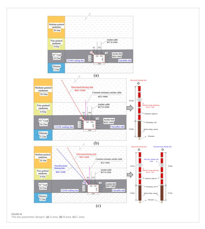
retained identical directional hole parameters while adding non-directional blast holes (33 m deep, 90 mm diameter, 50° inclination, 19.8 m charge length, 13.2 m grouted seal, Figure 16c). All holes utilized detonating cord initiation and were sealed with accelerated cement grout.
