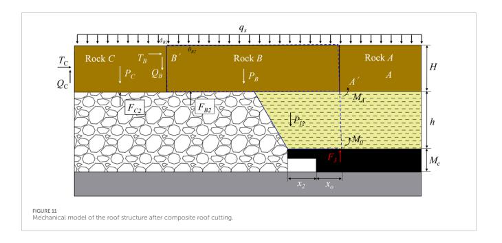
$$q_{s} \frac{L_{B}^{2}}{2} + M_{A'} + M_{0} + P_{B} \frac{L_{B}}{2} + P_{I} \frac{x_{1} + x_{0}}{2} - T_{B}(H - \Delta_{B}) + Q_{B}L_{B} - F_{1} \frac{2}{3}x_{0} = 0$$
