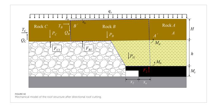
where  $M_c$  is the coal seam thickness, m; and h is the immediate roof thickness, m.
