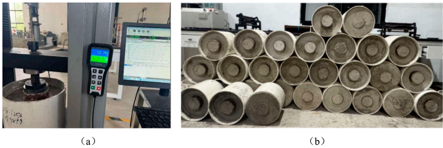
FIGURE 2 Interface contact test between the steel pipe and cemented soil pile. (a) Axial loading test (b) Samples made in the laboratory.
