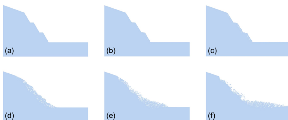
FIGURE 15 Deformation and failure processes of the terraced loess slope during rainfall. (a) step 0; (b) step 40000; (c) step 75000; (d) 130000; (e) 215000 and (f) 405000.
