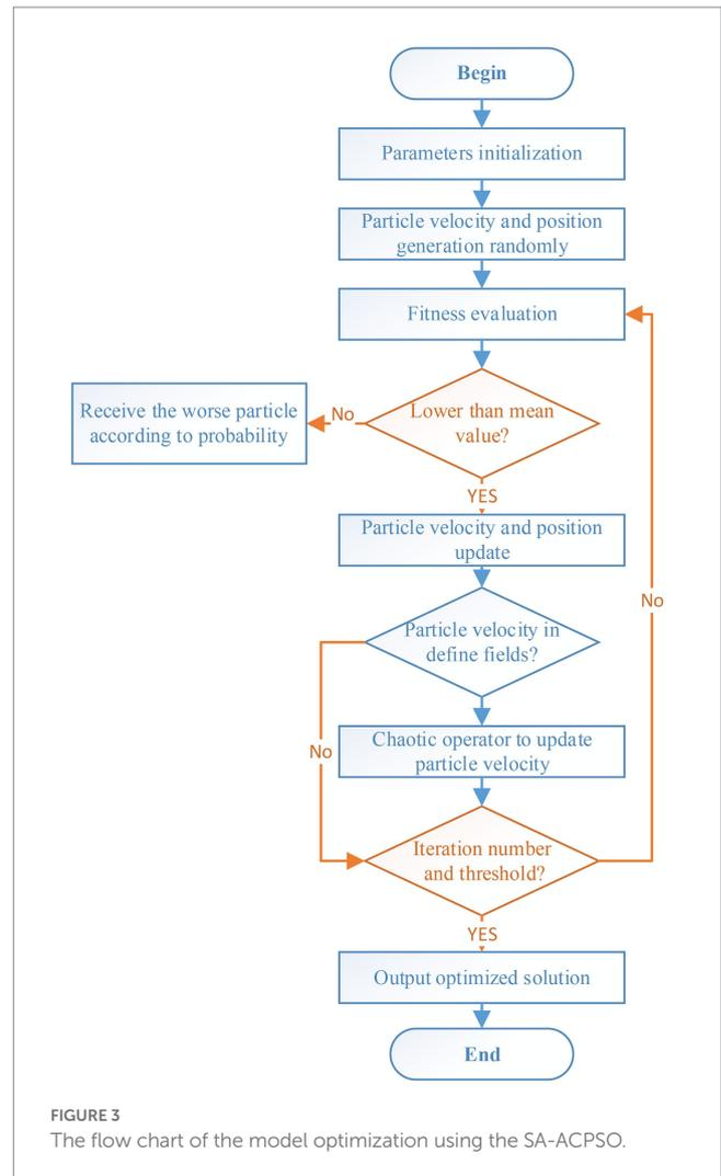
FIGURE 3 The flow chart of the model optimization using the SA-ACPSO.
