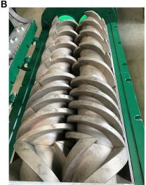
FIGURE 1 | A picture of the (A) The mini 3kW/h BioExtruder, (B) the counter rotating dual-screw auger from a commercial scale BioExtruder (model number MSZB 110e).
