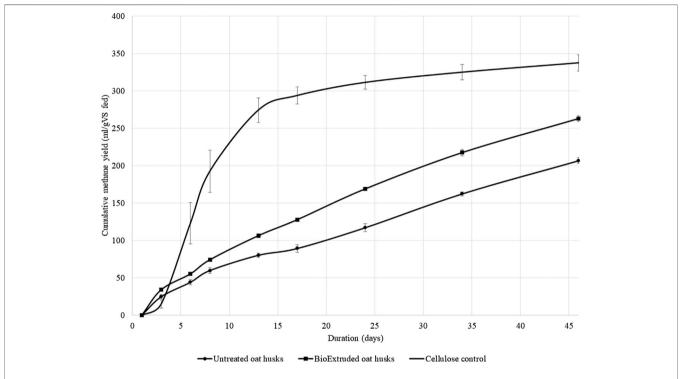
FIGURE 2 | The mean cumulative methane yield from oat husks (untreated and pre-treated via the BioExtruder) and cellulose controls. Digestate blank assay methane yields were subtracted from both treatment yields.
