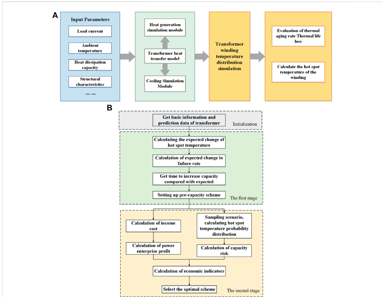
FIGURE 2 Online evaluation model and calculation process for load capacity assessment. (A) Online evaluation model for load capacity of oil-immersed power transformers, (B) calculation process of multi-risk transformer dynamic capacity increase strategy.
