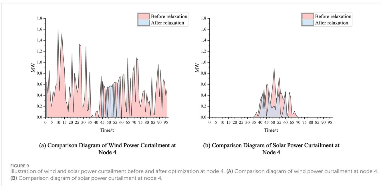
FIGURE 9 Illustration of wind and solar power curtailment before and after optimization at node 4. (A) Comparison diagram of wind power curtailment at node 4. (B) Comparison diagram of solar power curtailment at node 4.
