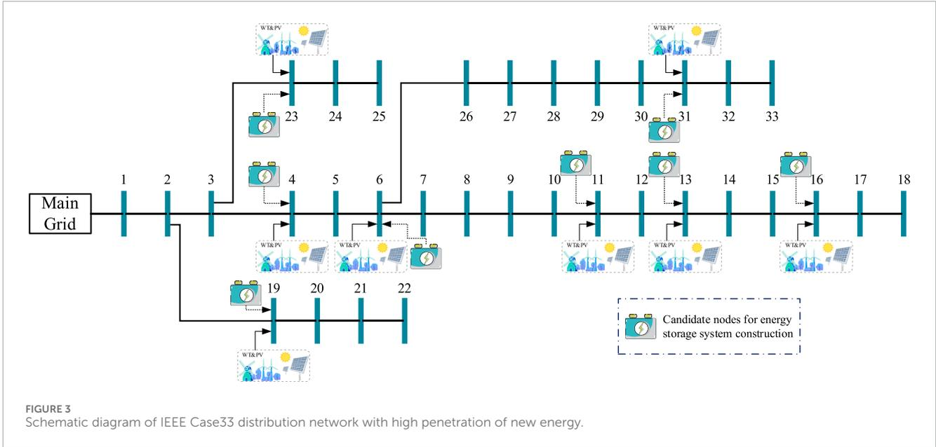
FIGURE 3 Schematic diagram of IEEE Case33 distribution network with high penetration of new energy.
