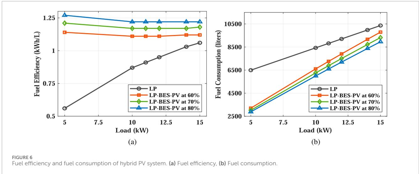
FIGURE 6 Fuel efficiency and fuel consumption of hybrid PV system. (a) Fuel efficiency, (b) Fuel consumption.
