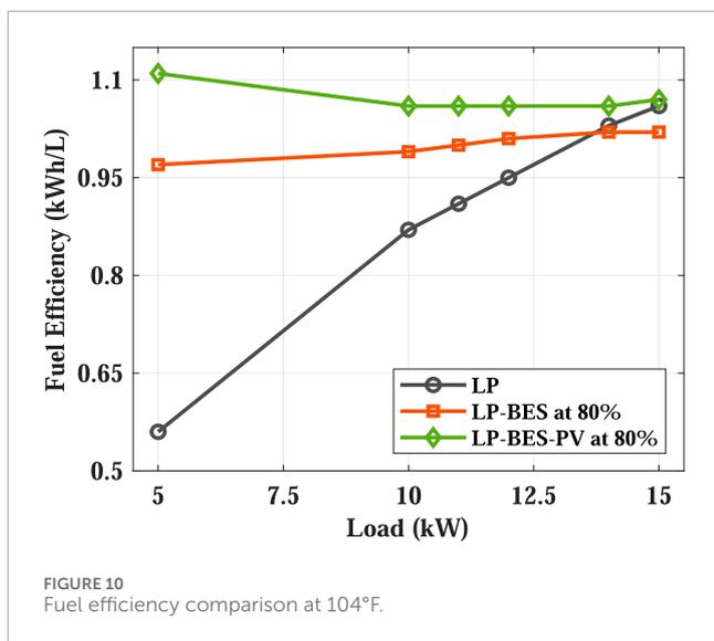
when the HPS operates with five PV panels with the LP generator operating at 60% and 80% capability. However, the savings are negligible over a 20 year period.
