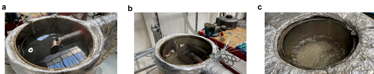
FIGURE 11 Level controls for system with an external cooker. (a) System with an external cooker (Figure 10a). Rotating a pipe bend for flow barrier control (Figure 10a). (b) System with an external cooker (Figure 10a). Displacement body for level control. (c) System with an external cooker (Figure 10a). Boiling water on the heat storage. The oil flow around the cooker is nonsymmetric, but boiling is quite uniform.
