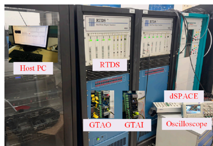
FIGURE 10 Topology of the experiment platform.
