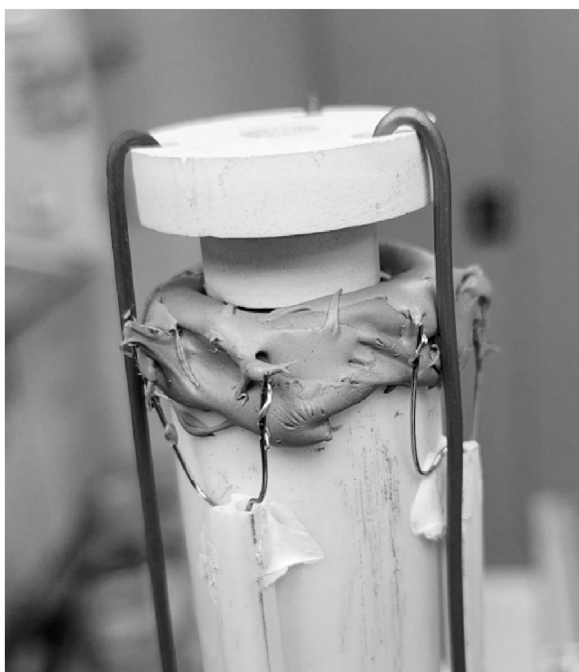
FIGURE 3 Assembled button cell, electrically connected to current leads and sealed to alumina test fixture. A ceramic air diffuser on the top is held with 3 spring-loaded metal wires.
