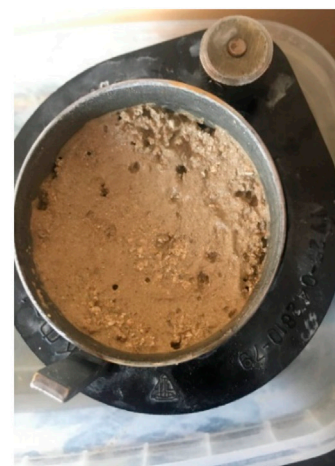
Manifestations of karst-suffusion process on the surface of the filtered limestone in KF-OOM
