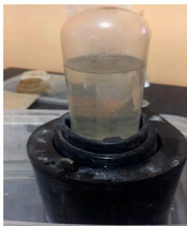
Water filtration in the Moriot flask of the KF-OOM device through limestone
