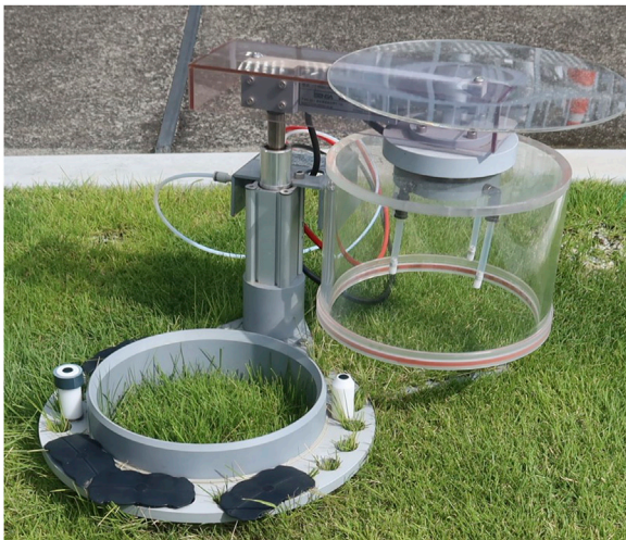
FIGURE 1 State of gas sampling from the thin-layer rooftop lawn on August 22, 2022. An automatic open/close chamber was set in the center of all turfs to measure the fluxes of CO 2 , CH 4 , and N 2 O from the surface of the rooftop lawn.
