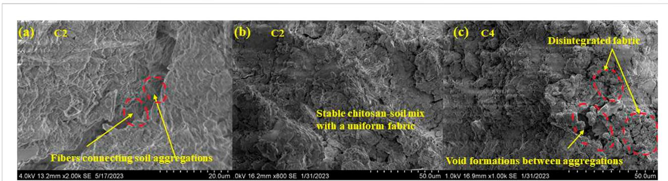
FIGURE 4 SEM images of the 90 days cured (A) C2 before durability test (B) C2 after fifth cycle (C) C4 after fifth cycle.
