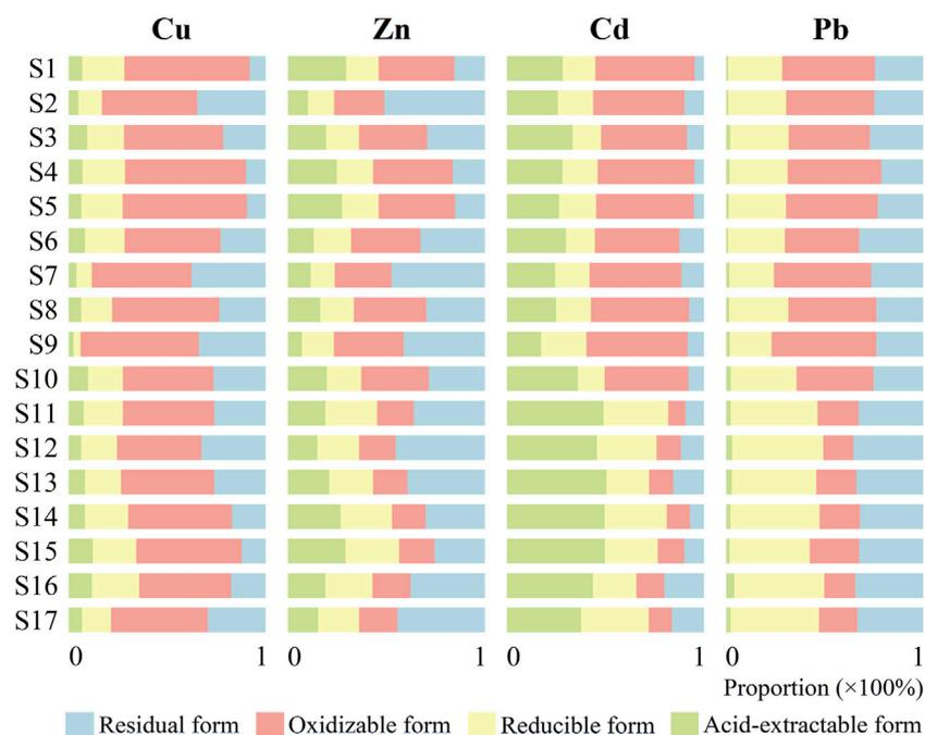
FIGURE 3 Percentage content of different chemical forms of Cu, Zn, Cd, and Pb in surface sediments.
