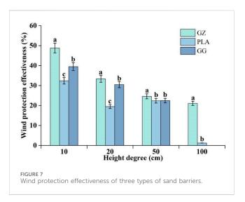
with the increasing vertical height and was lowest at 100 cm, while the weakening ability of PLA and GG sand barriers for wind was almost negligible.
