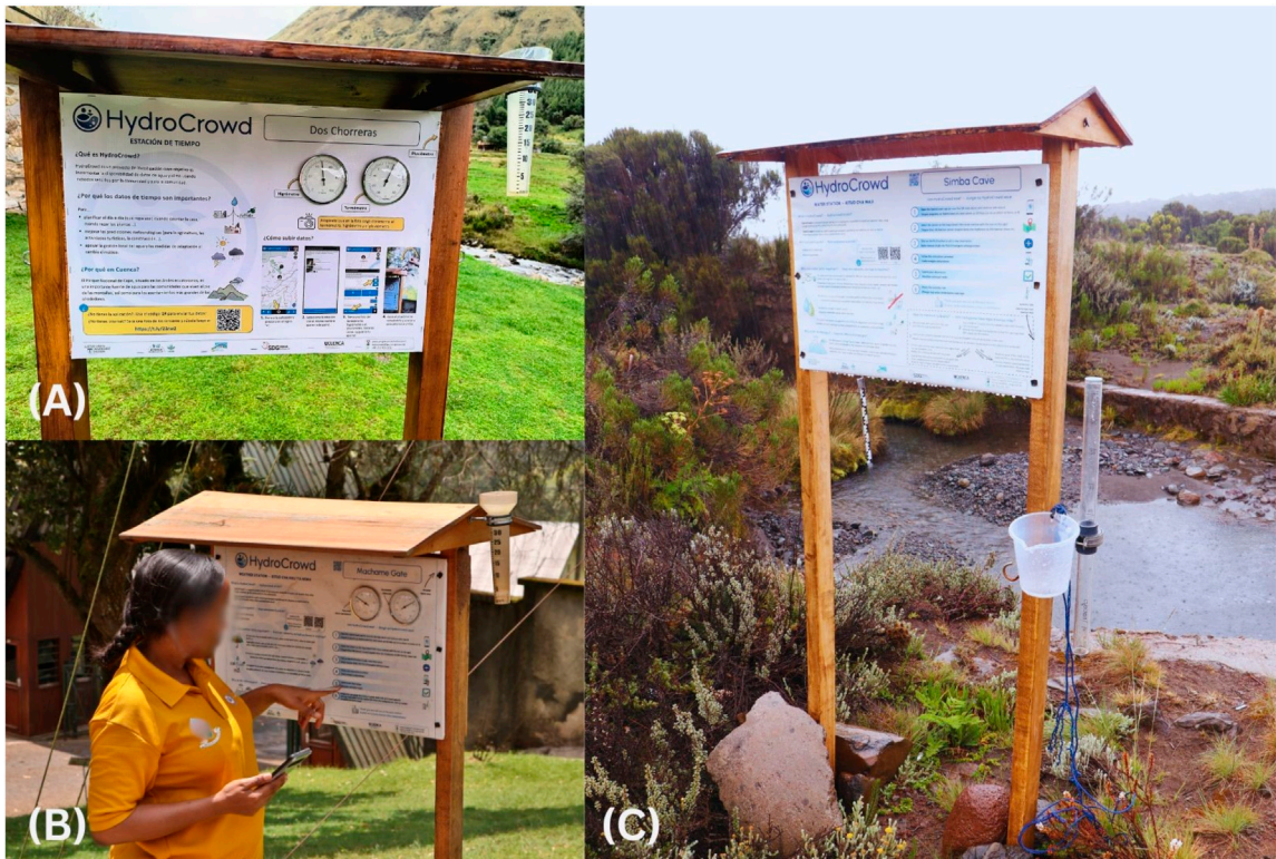
FIGURE 4 HydroCrowd stations. (A) Weather station in Cajas National Park. The panel features the provided instructions, the sensor installed, the rain gauge, and a QR code that can be used to submit data without downloading the app. (B) Weather station in Kilimanjaro National Park, which displays instructions for submitting data, which a volunteer can easily read. (C) Water station panel that includes a turbidity tube and a bucket for collecting water, as well as a water level gauge.
