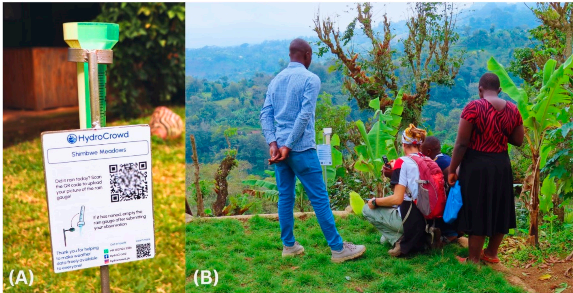
FIGURE 5 HydroCrowd weather@home stations around the Kilimanjaro National Park. (A) Close image of a weather@home station structure with instructions and the QR codes to download the app and submit data directly to the platform. (B) Volunteers collecting data from a weather@home station.
