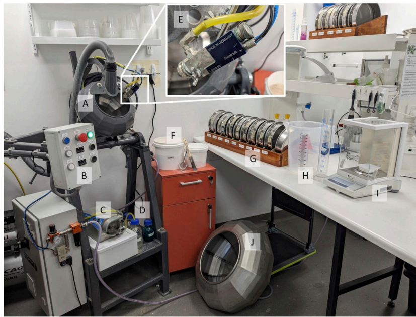
FIGURE 1 Seed pelleting station setup: (A) rotating pan, (B) control panel, (C) peristaltic pump, (D) liquid binders, (E) spray gun mounted on an adjustable arm, (F) fine powders, paintbrush and strainer, (G) set of sieves, (H) graduate volume cylinder (I), precision balance and, (J) larger replacement rotating pan. A list of items and costs is provided in Supplementary Material S1 .
