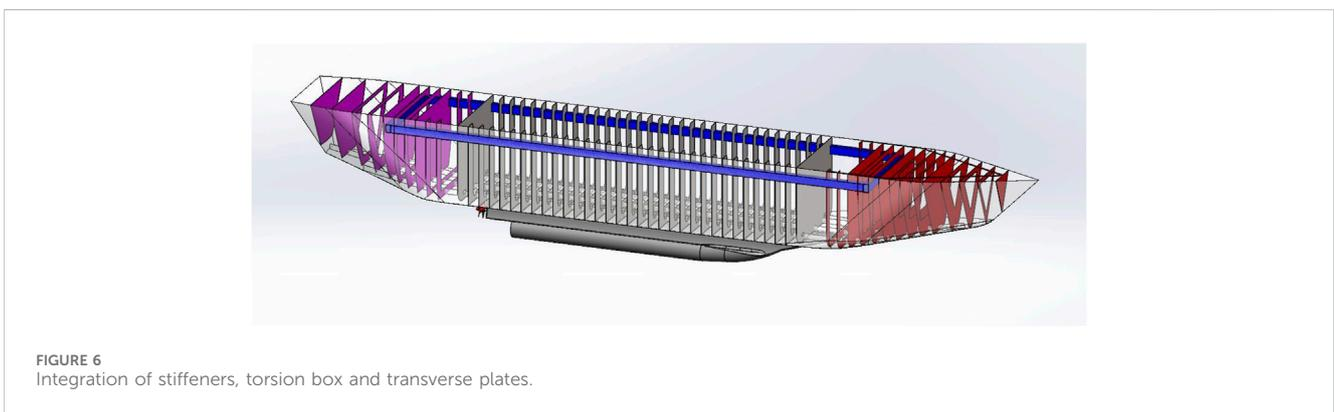
the centre of mass located 2.18 m below the deck. Stability analysis showed that the centre of gravity was located to the left of the metacentre when the ship tilted to the right, resulting in a stable vessel. The CAD model indicated that the keel had a surface area of 19.5 m<sup>2</sup>. The function relating vessel velocity ( $V_B$ ) and hull drag ( $F_{hull}$ ) is expressed in Equation 18.
