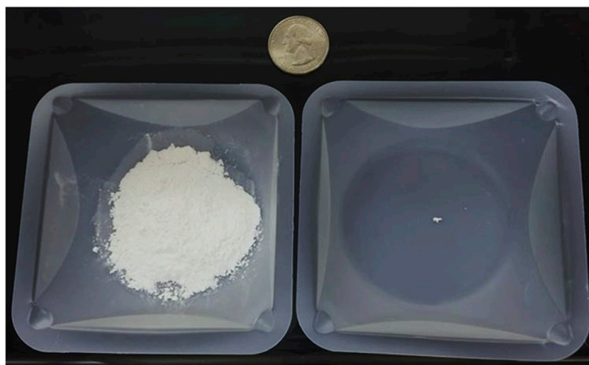
FIGURE 1 Starting materials of ~0.01% (100 ppm) asbestos (right) in coarsely ground talc chips (left). Further co-milling these materials together provides a thoroughly dispersed mixture with maximum homogeneity, simulating a production-scale ground mineral powder.
