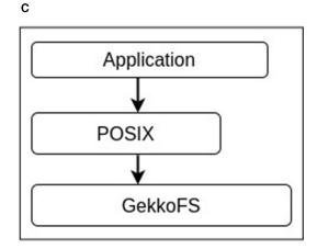
Examples I/O stacks to discuss the transport of I/O semantics. (a) Example I/O stack (Stack 1) using HDF5 and MPIIO as middleware on top of POSIX and Lustre. (b) Example I/O stack (Stack 2), where the application directly uses POSIX on Lustre. (c) Example I/O stack (Stack 3), where the application uses POSIX on GekkoFS.
