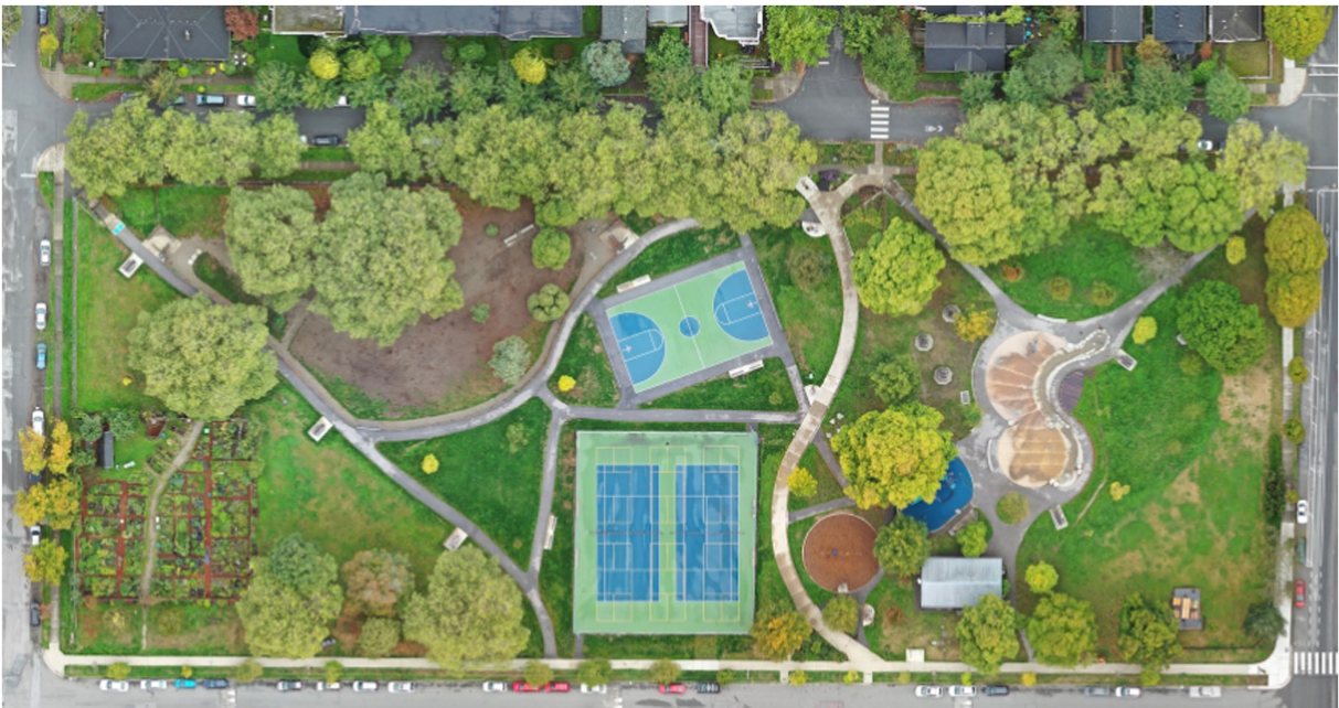
FIGURE 3 Orthomosaic generated from drone data collected at Pandora Park.
