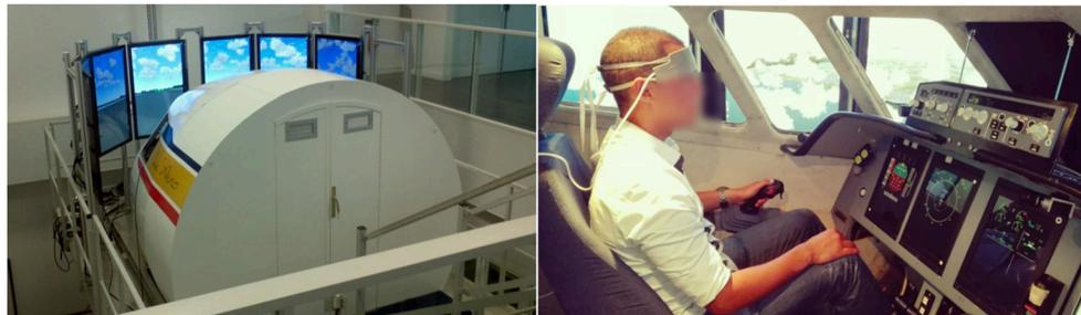
**FIGURE 2** | (Left) ISAE-Supaero flight simulator; the closed cabin is visible from rear, and eight screens are used to visualize external environment. (Right) The pilot subject with the fNIRS headband.
