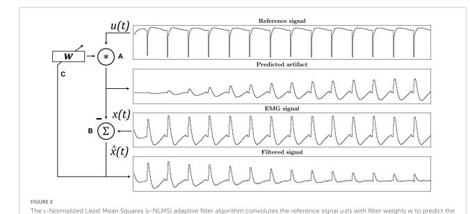
artifact waveform (A). The predicted artifact is subtracted from the original signal x(t) to yield an estimated artifact-free signal  $\widehat{x}(t)$  (B), which is
