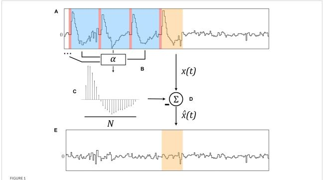
The Template Subtraction (TS) algorithm identifies stimulation artifacts from the original signal x(t) [(A), in blue] immediately following neurostimulation [(A), in red] and averages them using exponential filters (B) to form an artifact template (C). This template is subtracted from a newly-identified artifact [(D), in orange)] to yield an estimated artifact-free signal  $\hat{x}(t)$  (E).
