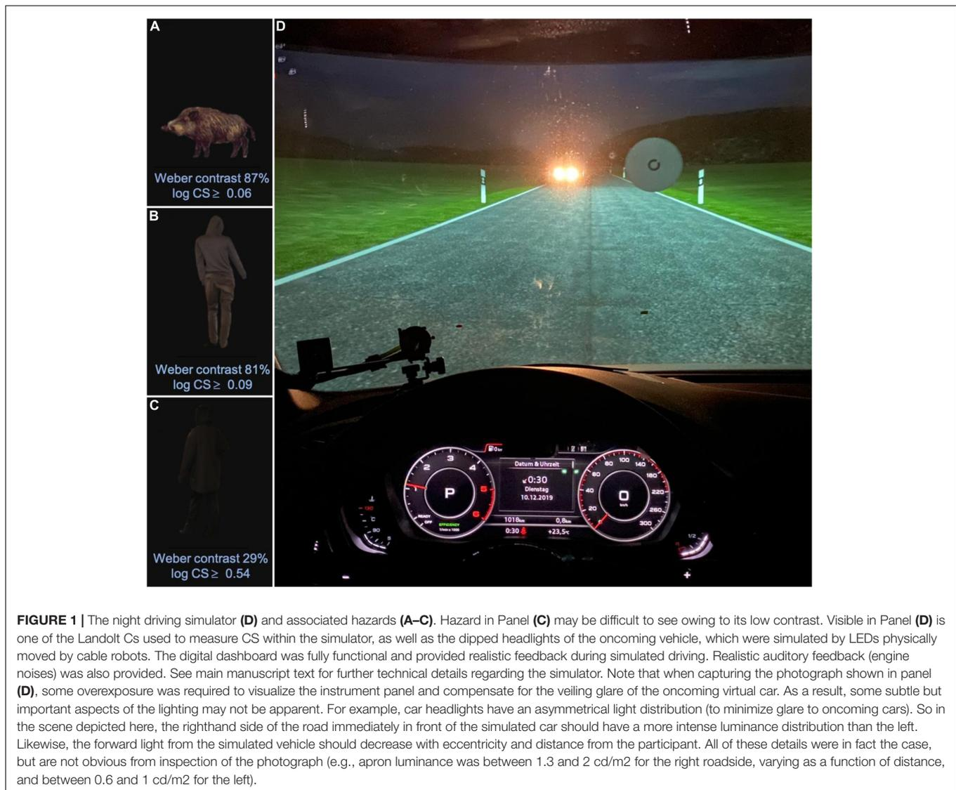
This confirmed that the luminance characteristics of the simulated scene corresponded, to a reasonable level of approximation (maximum deviation: 20%), to the on-road conditions of a vehicle with dimmed halogen headlights (Golf VII, Volkswagen AG).
