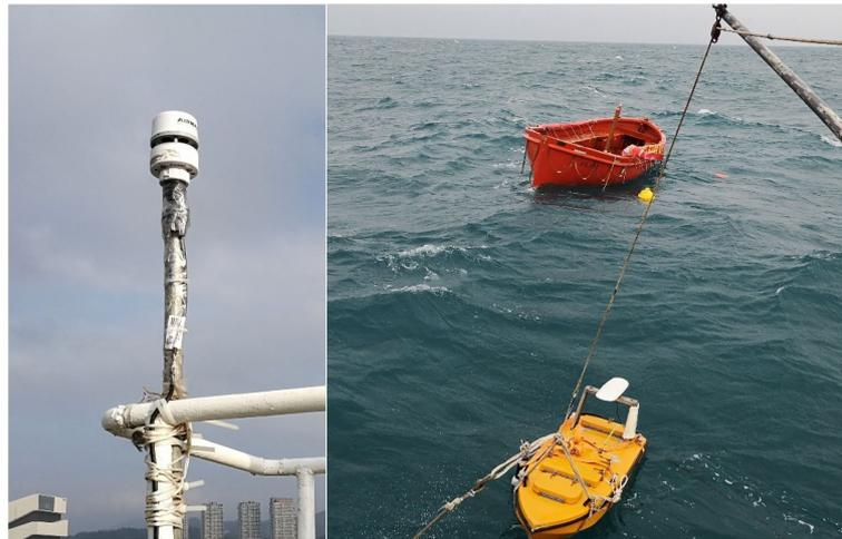
FIGURE 3 Installation of AirMar 220WX weather station (left), Nortek AquaDopp ADCP, Nortek Signature ADCP and GPS receiver (right).
