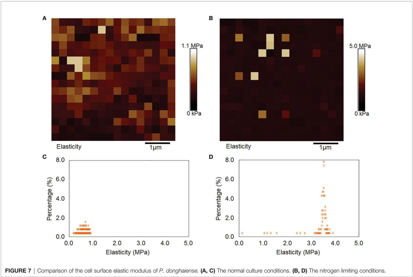
**FIGURE 7** | Comparison of the cell surface elastic modulus of *P. donghaiense*. **(A, C)** The normal culture conditions. **(B, D)** The nitrogen limiting conditions.
