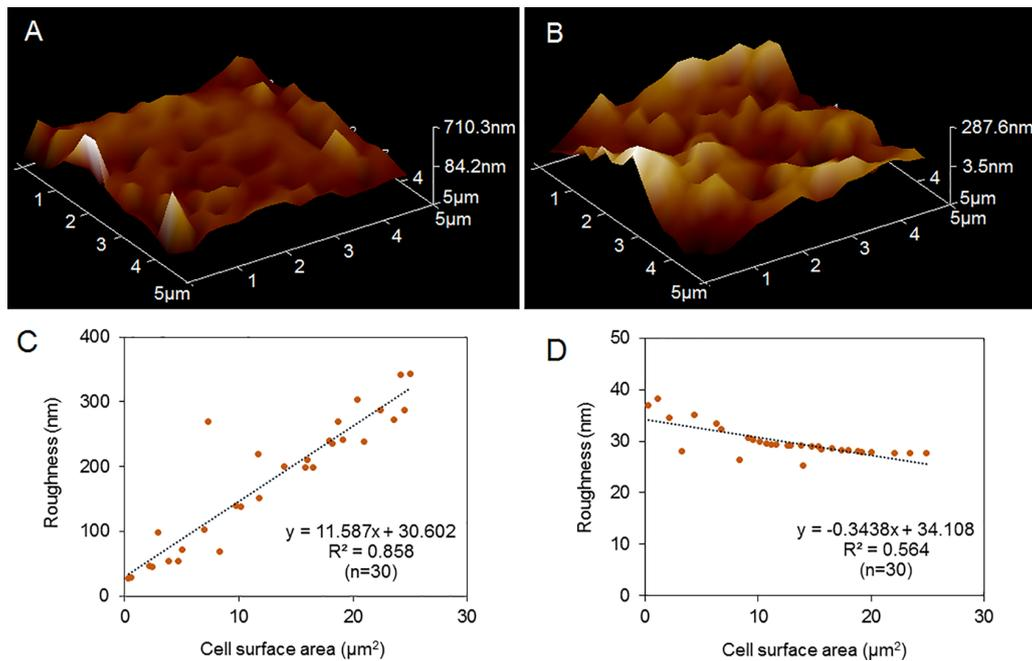
**FIGURE 5** | Comparison of the cell surface roughness of *P. donghaiense*. **(A)** 3D morphology of *P. donghaiense* under normal culture conditions. **(B)** 3D morphology of *P. donghaiense* under nitrogen limiting conditions. **(C)** Statistical analysis of roughness under normal culture conditions. **(D)** Statistical analysis of roughness under nitrogen limiting conditions.
