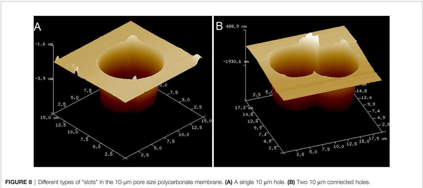
**FIGURE 8** | Different types of “slots” in the 10-µm pore size polycarbonate membrane. **(A)** A single 10 µm hole. **(B)** Two 10 µm connected holes.
