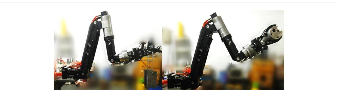
FIGURE 11 Physical view of the manipulator when grabbing 50kg and 10kg heavy objects respectively.
