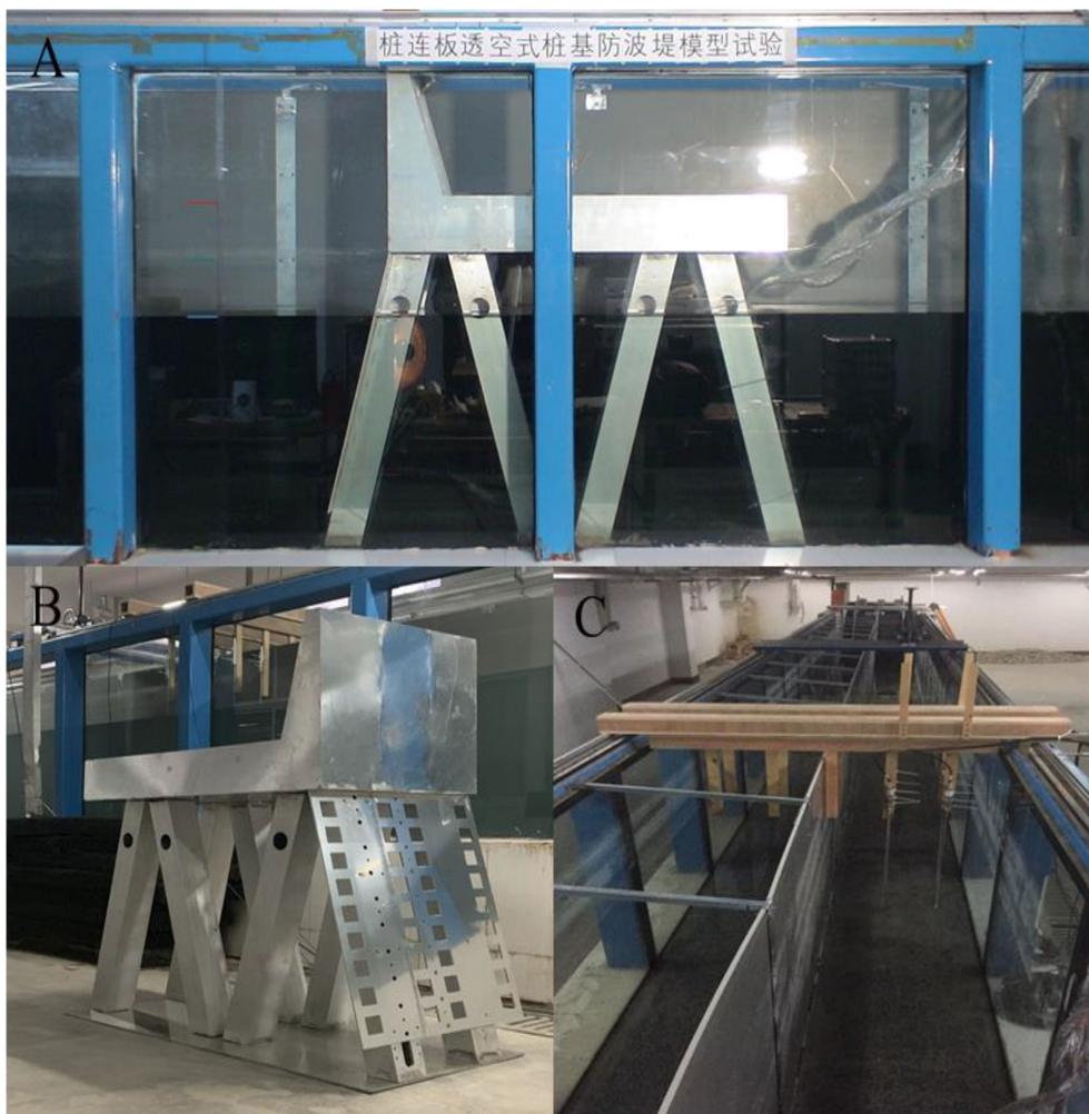
**FIGURE 3** Experimental set-up in the hydrodynamics laboratory: (A) arrangement of the model in the wave flume and (B) model of breakwater for testing, and (C) the fixed bulkhead.
